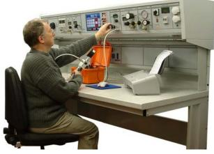
**CalBench** is the ultimate multifunction calibration station from Time Electronics. A wide range of standard modules can be mounted in the primary console; this gives a highly flexible system that is both functional and easy to use. Further expansion can be achieved by adding the optional secondary console 7081.
